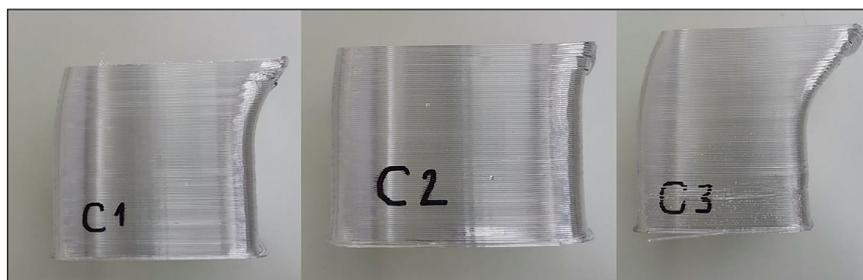
**Figure 1.** Samples with overhang defect as result of planar slicing
