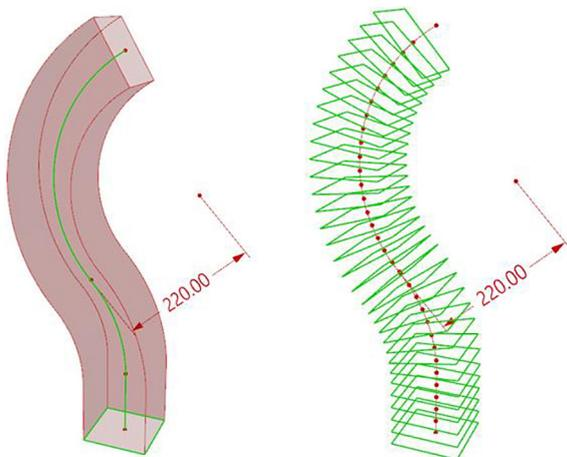
Figure 4. Curve led planes generation and intersection
