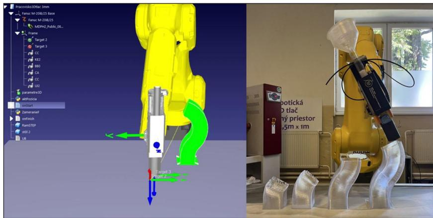
Figure 7. Simulation in RoboDK software (left) and test samples printing process (right)
